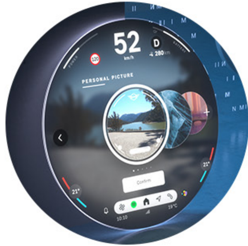
MINI Interaction Unit: Round Central Unit with an Area of 440 cm 2 (9.4 inch) with OLED Technology.
