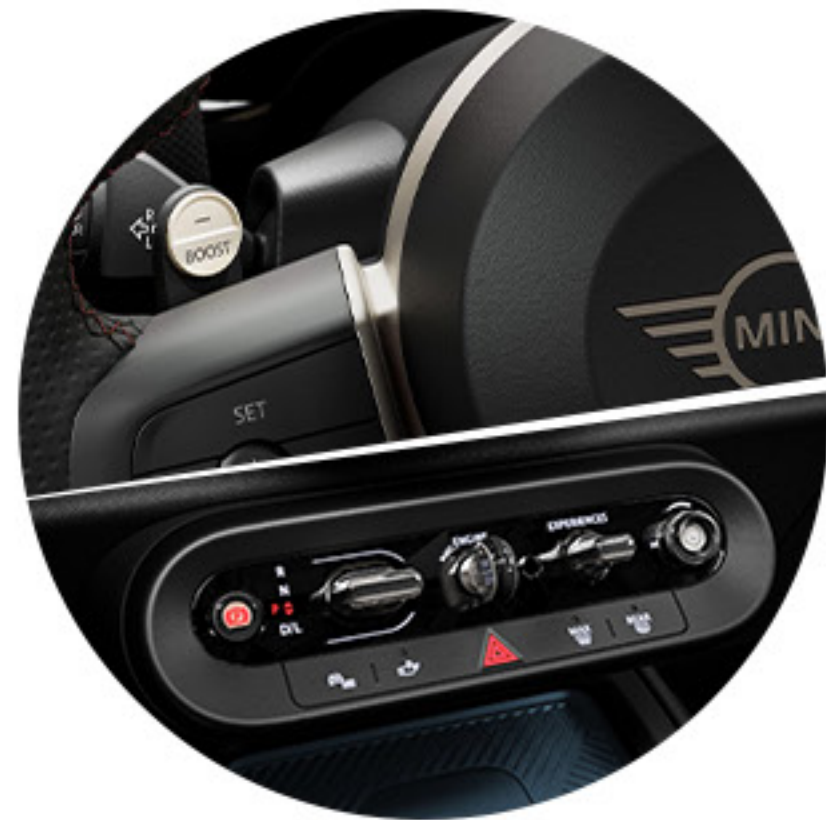
Steptronic sport transmission with gearshift paddles (Only for S & JCW Engines).
