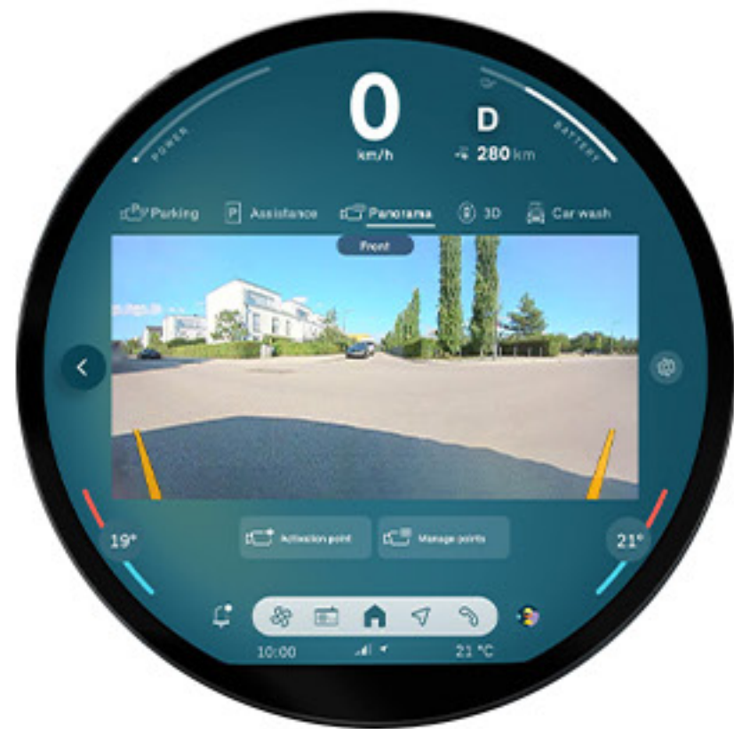
Parking Assistant Plus: Visual parking aid featuring Surround View cameras, Top View, Panoramic View and 3D View makes parallel and perpendicular parking on the road easier. The system completely takes over the steering, the accelerator, and the transmission.
